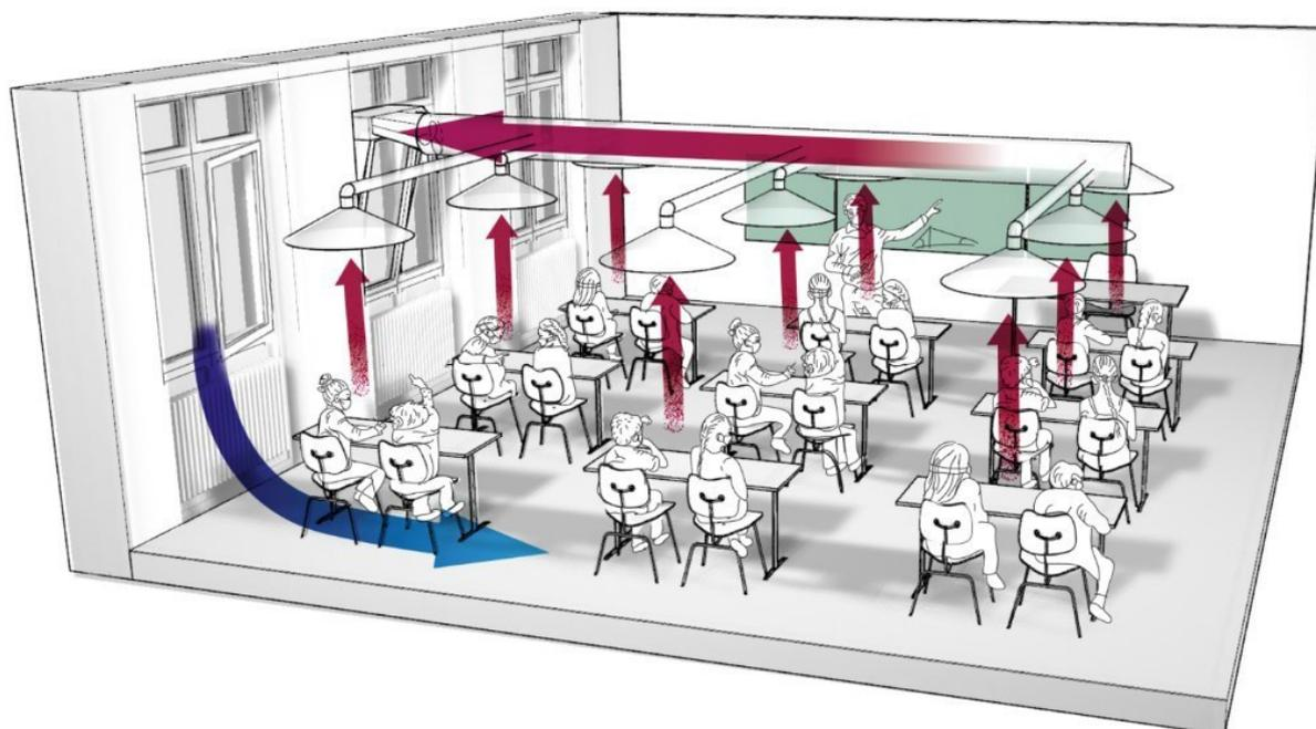
**Figure 4:** Schematic diagram of a mechanical extract ventilation system with distributed extract ducts and hoods (MPIC-MEV hood version) ([ventilation-mainz.de](http://ventilation-mainz.de)).
