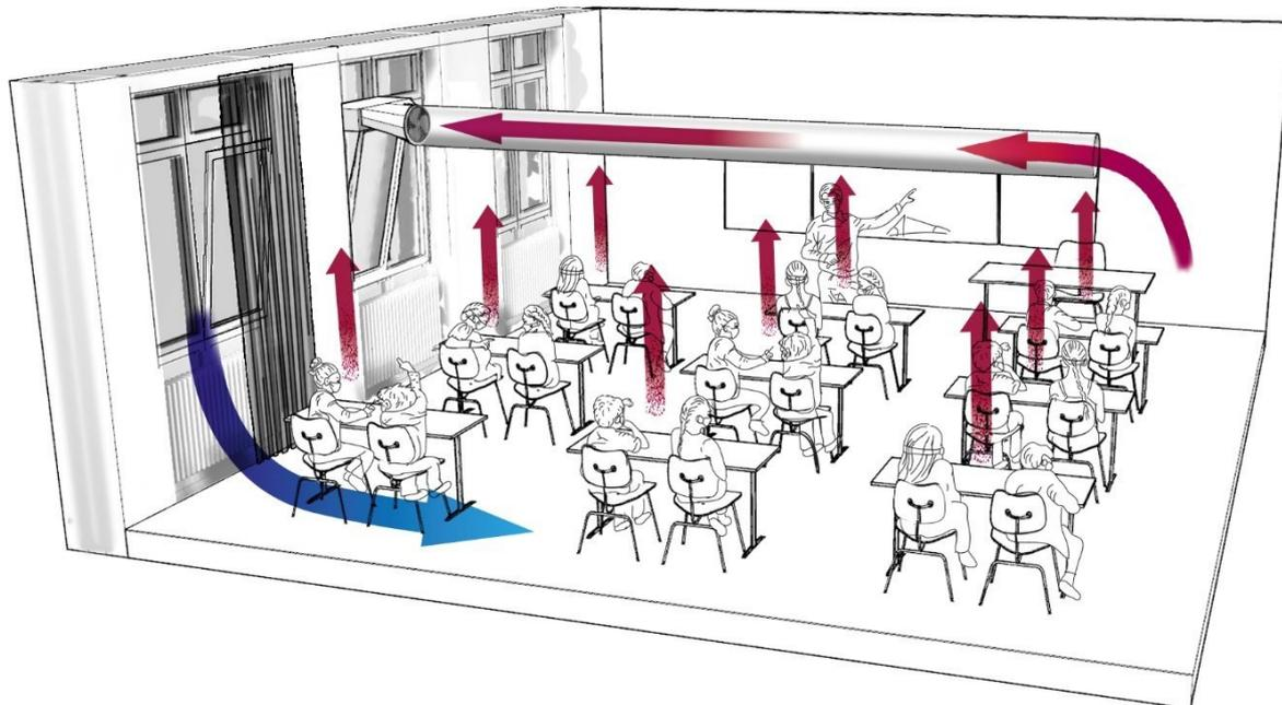
**Figure 3:** Schematic diagram of a mechanical extract ventilation system with central extract duct (MPIC-MEV base version) ([ventilation-mainz.de](http://ventilation-mainz.de)).
